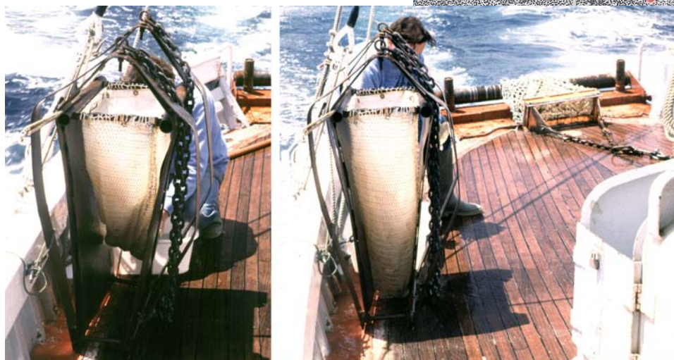
Figure 2-5 : Epibenthic sledge being collected from the sample (left) and ready for the next launch.
