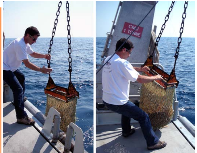
Figure 2-2 : Return to the deck of a Charcot-Picard dredge without underpants (Photos taken from a video).
