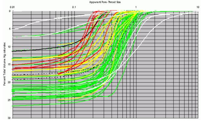
**Figure 7:** Hg injection data: "apparent pore-throat-size" (µm) versus "total volume Hg saturated" (%), cumulative. These should be histograms; curves are used only for display!
