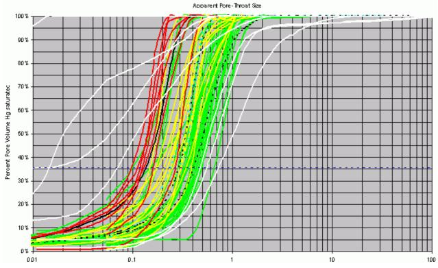
**Figure 6:** Hg injection data: "apparent pore-throat-size" (µm) versus "pore volume Hg saturated" (%), cumulative. Dashed horizontal line at 35% Hg injection. These should be histograms; curves are used only for display!
