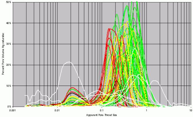
**Figure 5:** Hg injection data: "apparent pore-throat-size" ( $\mu$ m) versus "pore volume Hg saturated" (%). Key: red for R-chalk ("B"); yellow for RR-0.25 ("C"); green for RR-0.45 ("D-E"); white for discarded samples. These should be plotted as histograms; curves are used only for display!
