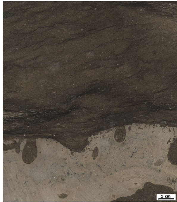
Figure 9: Scan of polished core (slab). Hard-ground marking the Lekhwair-Kharai boundary in well N° 19.
