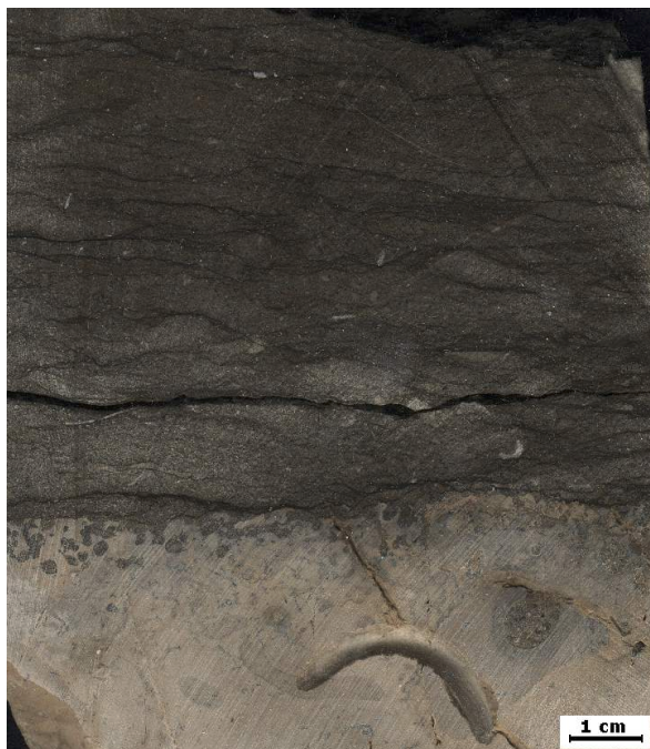
Figure 8: Scan of polished core (slab). Hard-ground marking the Lekhwair-Kharai boundary in well N° 12.
