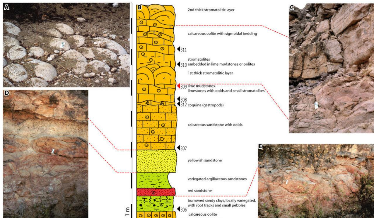
**Figure 2:** **A)** Stromatolitic domes capping the section; **B)** schematic lithologic log of the quarry section (Yacoraite Formation) with the location of the sampling points; **C)** first thick stromatolitic layer (8.5-10 m) overlain by oolitic facies; **D)** the yellowish sandstone (3-4.5 m) overlying a variegated argillaceous sandstone; **E)** the red sandstone (1.5-2 m) overlying variegated sandy clays.
